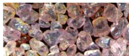
Weak Indian Garnet particles with fracture lines
